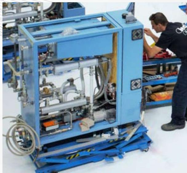
Available version "G" with heating system by Methane Gas or LPG (Ieci patent)
